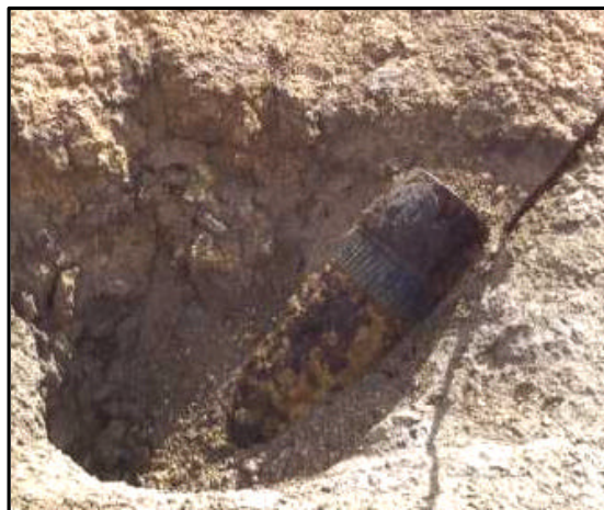
Partially Exposed 5-inch Projectile
