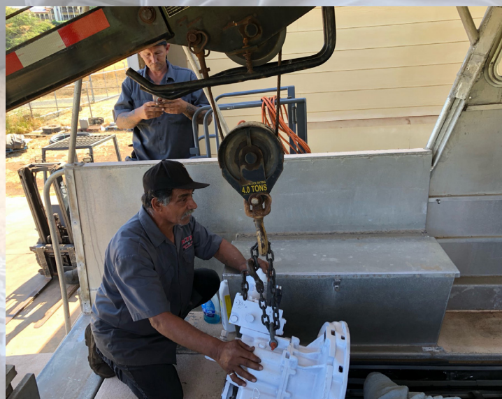
▲ Mechanic is lowering and installing the rebuilt transmission
