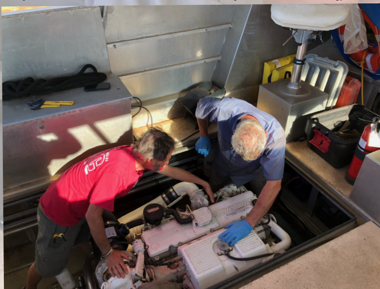
▼ KIRC staff Grant Thompson working with a mechanic to re-couple the port side transmission with the motor after it was rebuilt off-site
