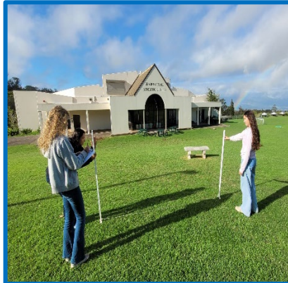
Photos Above: Seabury Hall marine science students learn how to measure beach slope change using the Emery method and then are shown how to plot their measurements in a graph.
