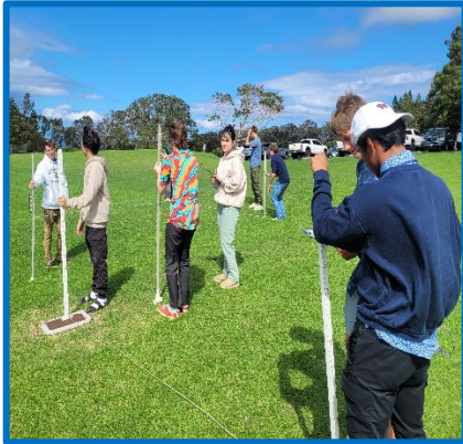
Photos Above: Seabury Hall marine science students learn how to measure beach slope change using the Emery method and then are shown how to plot their measurements in a graph.
