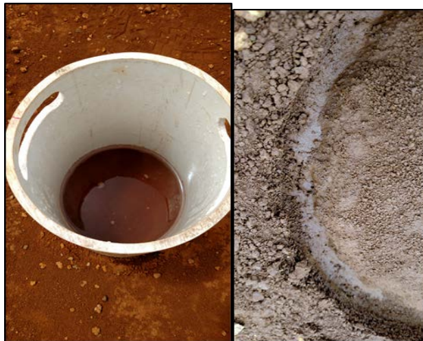
Measuring soil infiltration in hard pan soils (non-restored). Note no roots. (Photos by James Bruch)
