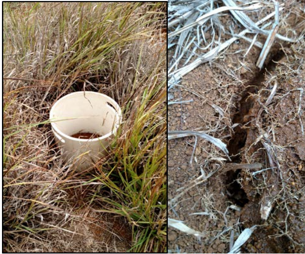
8" PVC pipe measuring soil infiltration in Pili grass (restored). Note roots in soil.
